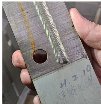
Stainless steel test 1,467 days
